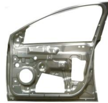
Figure 25: Door Inner Finished
