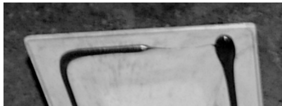
Figure 8: Example of a "Tail" and "Blob" at the End and Beginning, Respectively, of a Dispense Pattern
